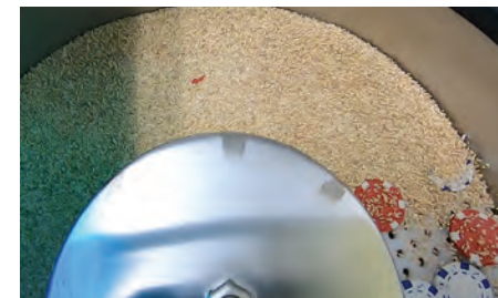
Chips and dice pass through hot organic granulate.
